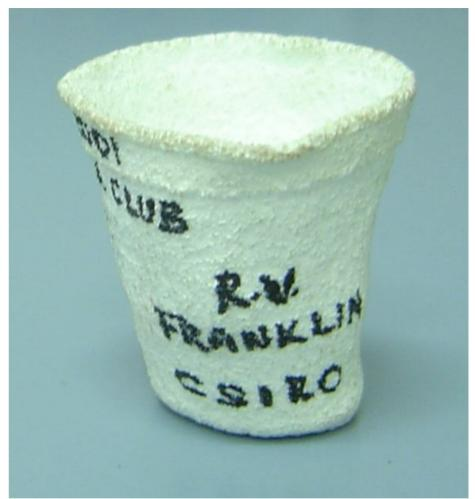
A polystyrene cup after it came back from the depths of the Pacific Ocean. The air inside the bubbles has been forced out, collapsing the cup.
